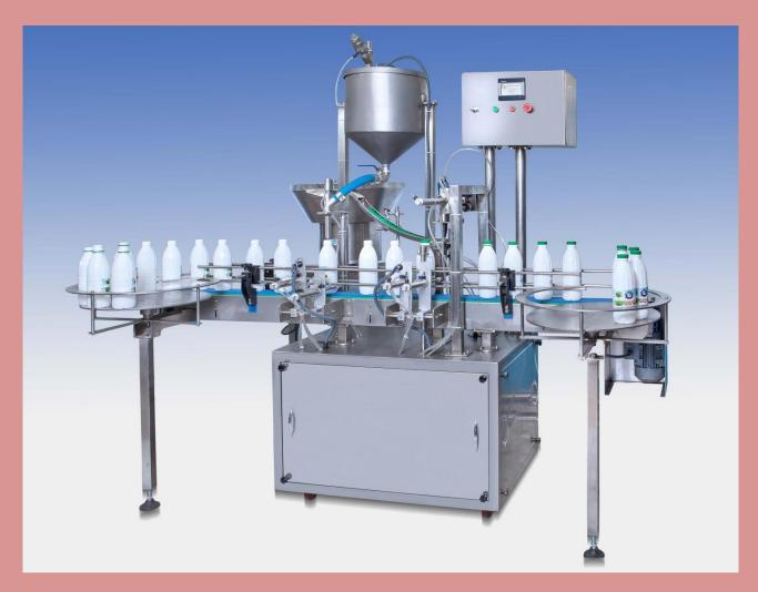
Plastic bottle filling and sealing machine works with a mechanical gearbox and a linear moving system. It is possible to fill variety of plastic bottle sizes. Bottles lined on the conveyor belt are capped at the lid station and accumulated on the output tray ready for packaging.
